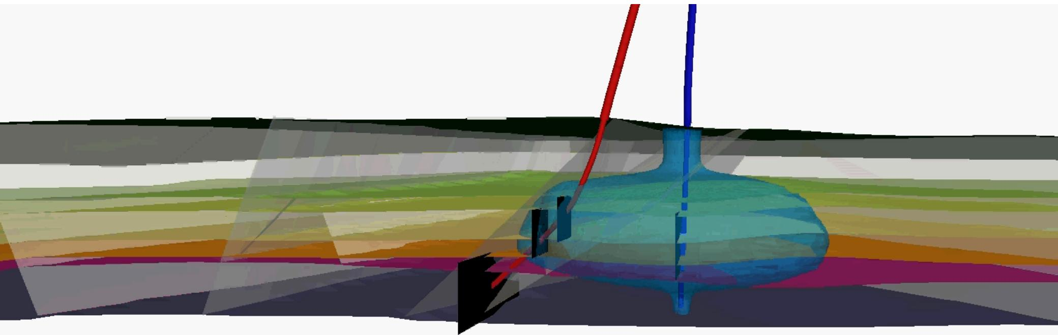
Propagation of cold water front ( $135^{\circ}\text{C}$ ) around the injection well ( $75\text{m}^3/\text{h}$ ;  $70^{\circ}\text{C}$ ) over a period of 30 years
