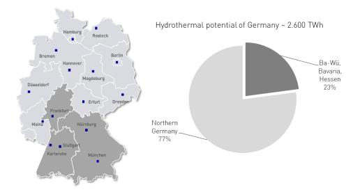
Figure 17 Geothermal exploitation in Germany: Distribution of the technical potential of hydrothermal systems between the Northern and Southern part.
