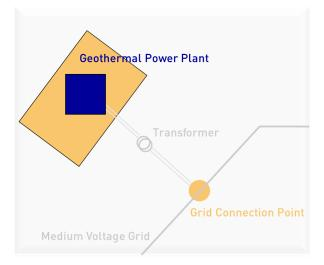
Figure 20 Allocation of the grid connection point. Best-case-scenario: connection of the power plant to electricity grid by using the shortest distance (linear distance).
