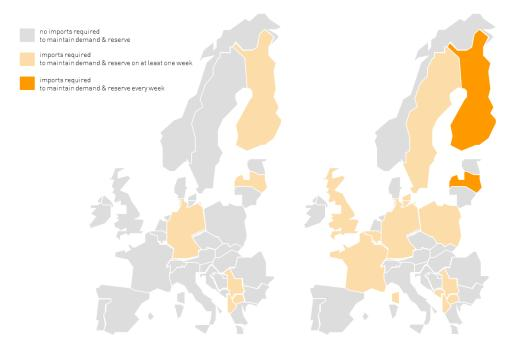
Figure 8 Country analysis under normal conditions (left) and severe weather conditions (right) (ENTSO-E, 2011)
