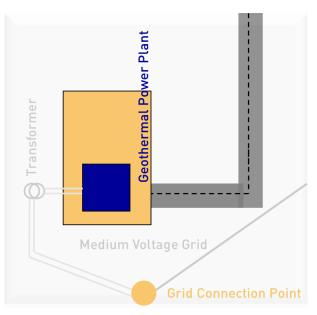
Figure 22 Allocation of an alternative grid connection point. The nearest (linear distance) grid connection point is unsuitable due to economic issues.
